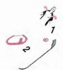
7 Pull the red handle to reveal the electrode pads.
