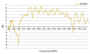
$<sup>^4</sup>$  Measured connected directly to IBflex $^8$  scanning receiver, which provides a ground plane of 4.4" x 1.55" (112 mm  $\,$  x 39 mm).
