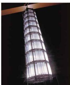
Artificial quartz crystal drawn from an autoclave
